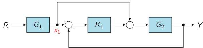
Add variables to the diagram at branch points. These are shown in red on the diagram above.
