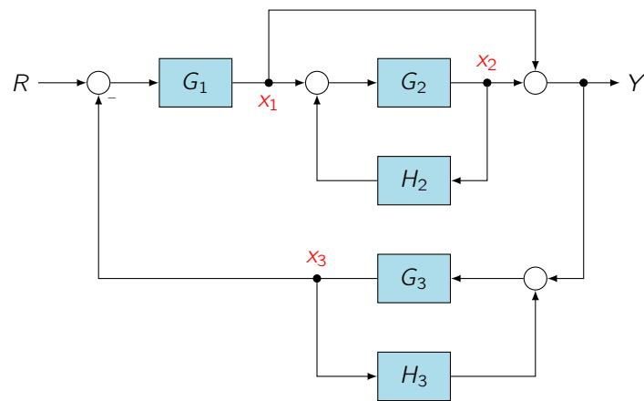
Add variables to the diagram at branch points. These are shown in red on the diagram above.
